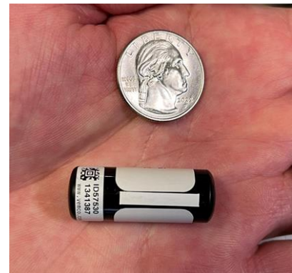
Figure 2. The Vemco V13 coded transmitter. These transmitters are 13 mm in diameter and 36 mm long.
