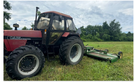
An enclosed cab is a safer option to protect against sap exposure while mowing.
