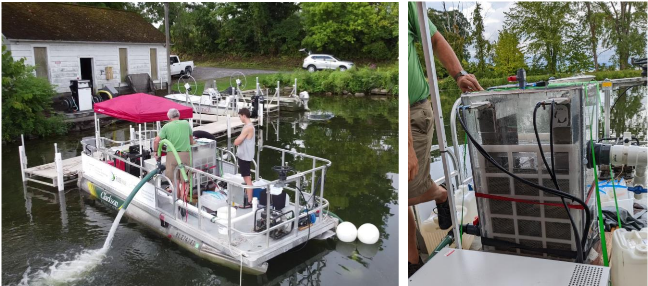
EO equipment in operation at 100 gallons per minute at Oneida Lake in 2022 (left). The electrochemical reactor vessel (right). Photo credit: Lewis McCaffrey
