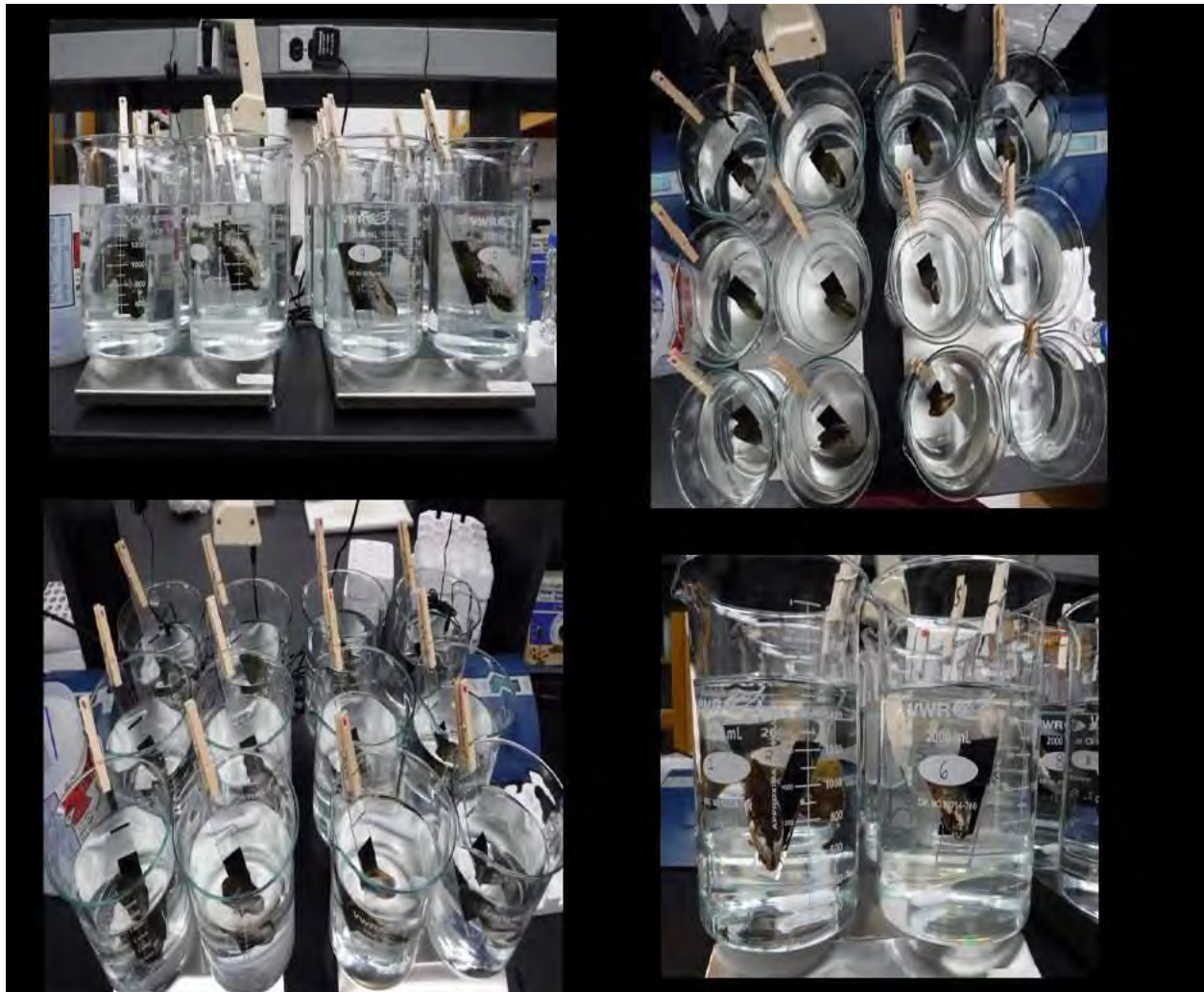
Figure 11. Experimental layout, with 12 beakers on magnetic stir plates each containing 1 mussel (either live or empty shell) attached via Velcro to a plexiglass strip held to beaker with a clothespin.
