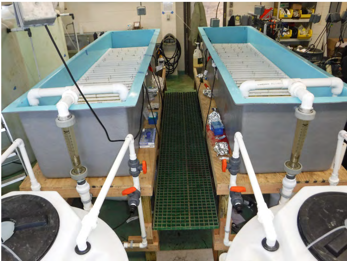
Figure 4-1 Experimental tank set-up with the header tanks shown in the foreground
