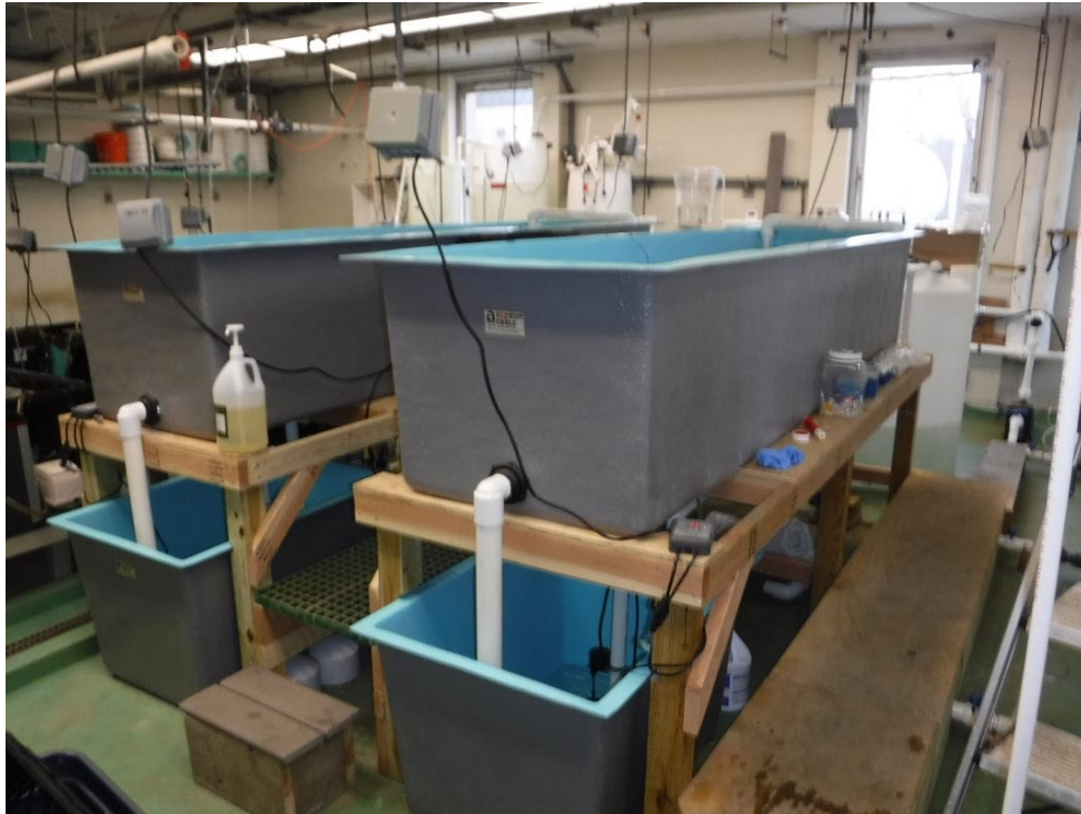
Figure 1-1: Experimental Tank Setup showing the Main tank the collector tank and the header tank (in the back)
