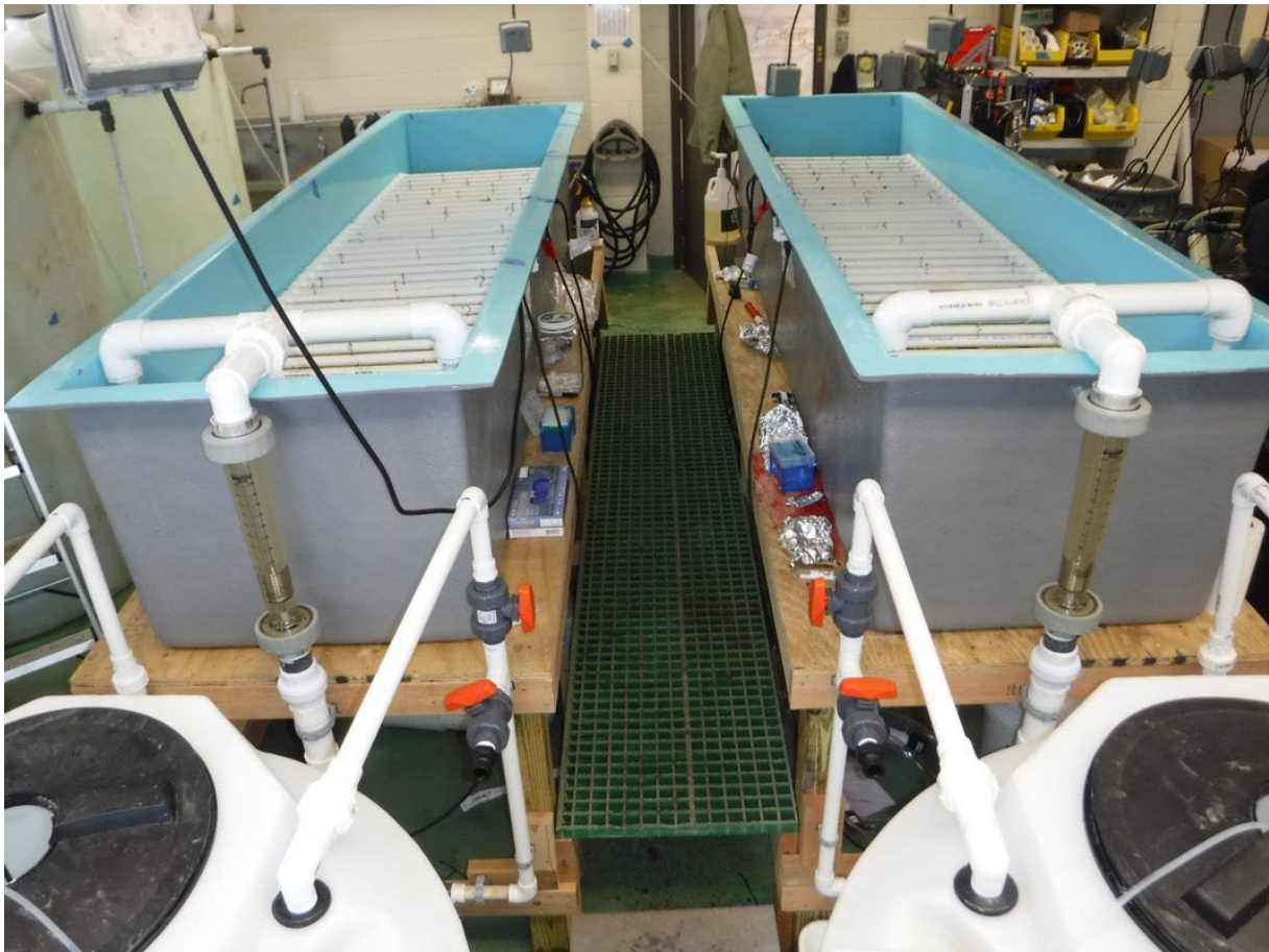
Figure 4-2: Experimental tank set-up with the header tanks shown in the foreground
